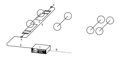
2. With more than one pair of scales axle groups can be measured in one operation.
