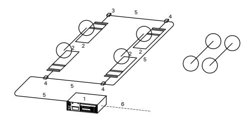
With more than one pair of scales a vehicle can be measured in one operation. The Number of axles to be measured at the same time is limited to 6.
